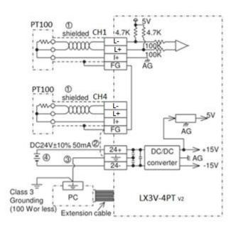
The cable of the PT100 sensor or a twisted shielded cable should be used for the analog input cable. This analog input cable should be wired separately from power lines or any other lines which may induce noise.
