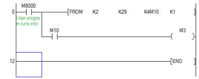
Transfer the error status to (M25 to M10), when error is found, M10=ON
