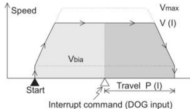
When the start command is received, the motor starts operation. When the INTERRUPT input is received, the motor moves by the specified distance, then stops (The relative travel exclusively can be specified.) The current value is cleared by the start command. The current value starts to change by the INTERRUPT input, and becomes equivalent to the set position when the operation is completed.
