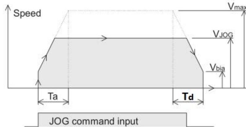
Any value between the bias speed  $V_{bia}$  (BFM #6) and the maximum speed  $V_{max}$  (BFMs #5 and #4) is valid as the command speed  $V_{JOG}$  (BFMs #8 and #7). When JOG signal continues to be 1 for less than 300ms, one reverse pulse is generated. When JOG signal continues to be 1 for 300 ms or more, continuous reverse pulses are generated.
