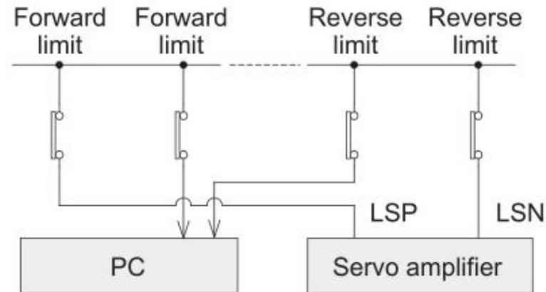
Because a drive amplifier for a stepper motor does not have these terminals, make sure to provide limit switches on the PLC.
