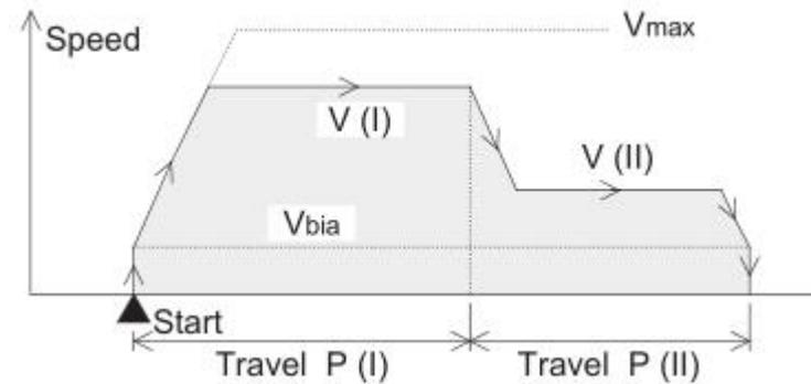
The motor performs the following operation by the two-speed positioning operation command. Approach at high speed as well as processing and moving forward at low speed can be performed. When the start command is received, the motor performs positioning at the operating speed  $V(I)$  (BFMs #20 and #19) until the set position  $P(I)$  (BFMs #18 and #17), then at the operating speed  $V(II)$  (BFMs #24 and #23) until the set position  $P(II)$  (BFMs #22 and #21) (two-step speed).
